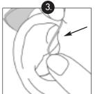
Step 3: While holding the receiver module in place in the ear canal with your thumb or index finger; carefully place the hearing instrument body over the top of your ear
