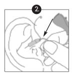
Step 2: At this point, the instrument is inverted from its final position. Carefully insert the receiver module into the ear canal. Make sure the locking wire is located inside the bowl of
